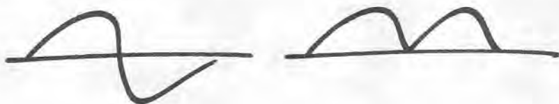
Figure 8: Sine curve with the negative part folded upwards, leading to a “metallization” of the sound.
